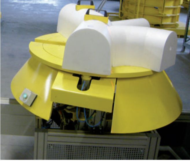
At VMC hot wire cutting is used to cut the material-saving EPS-mould parts to suit your project requirements; the picture shows the saw for shaping the berms.
